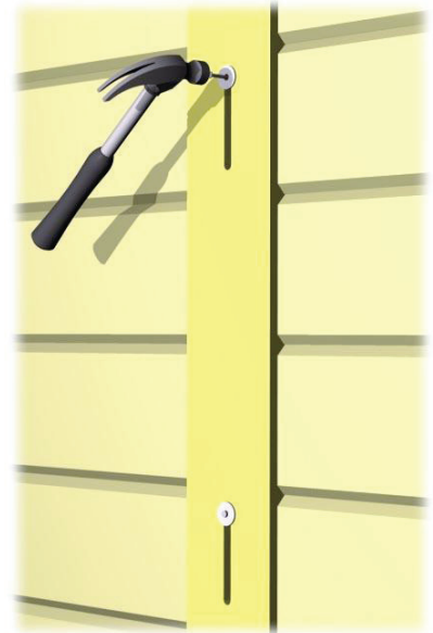
3. Fixing the stud of the interior wall in the groove
