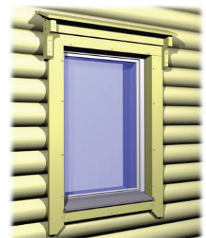
6. Architraves in a round log wall
