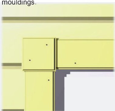
5. Nail the corner decoration pieces to the mouldings. Use brads with a length of 40 mm at most.
