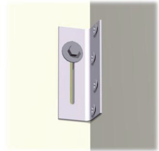
3. Fix the sliding angle bracket with a head bolt or other sturdy screw to the log at the top edge of the long hole and to the cupboard wall with 15x4 screws.
