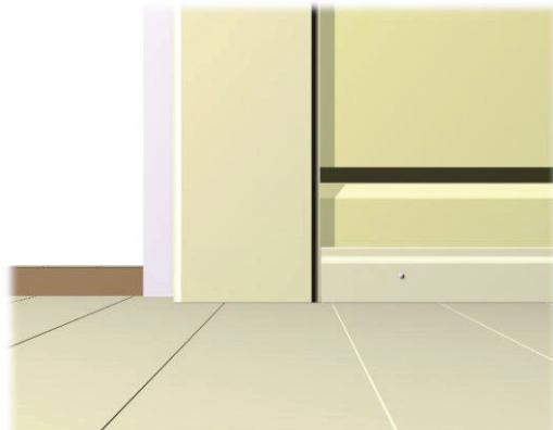
3. Connection of moulding to door frame board
