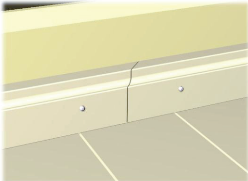
2. Extending a moulding.
