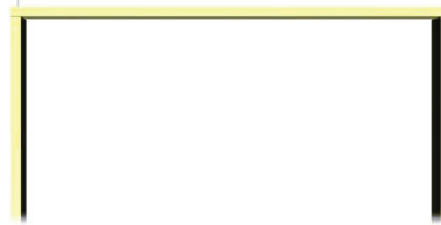
2. Nail the reveal liner of the upper side to the side liners.
