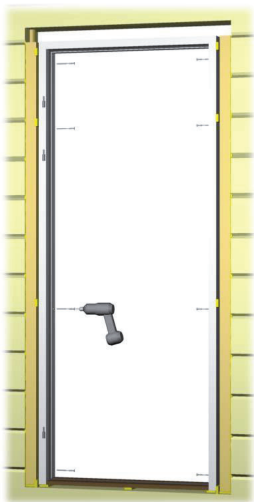
1. Installing the frame of the entrance door
