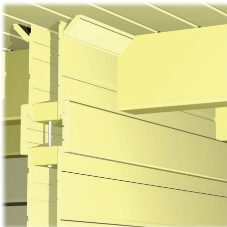
4. The figure illustrates mouldings for the settling space where beams penetrate the wall when the intermediate floor beams remain visible
