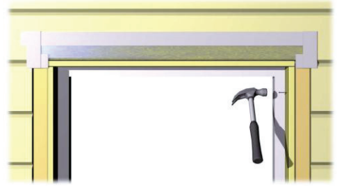
3. Nail the reveal liners on both sides to the jamb plank.
