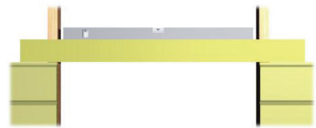
2. Monitoring panelling height on both sides of the door opening.
