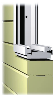
5. Rectangular/laminated log wall
