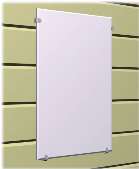
5. Fixing a large mirror on a log wall. The mirror rests upon lower brackets. The upper brackets allow for log wall settling.
