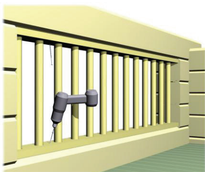
3. Lift the planks and spokes between the railing logs and nail or screw them
