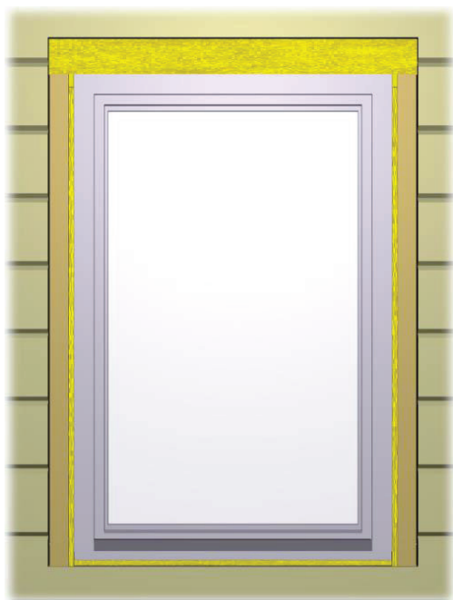
3. Finished frame insulation.
