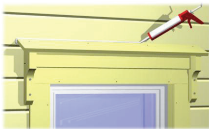
4. Upper architrave, top board and decoration piece. Sealing the top board with silicone
