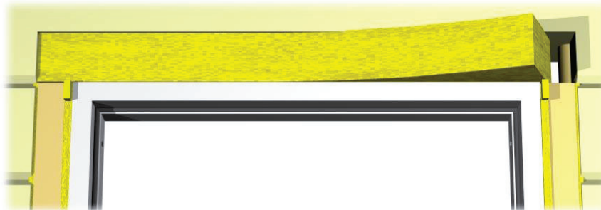
1. Insulation of the settling space above the door.
