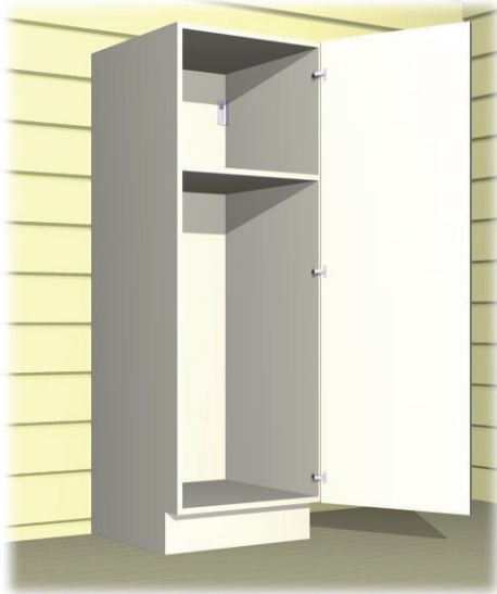
1. Fixing a high cupboard on a log wall. Mount sliding angle brackets inside the cupboard.
