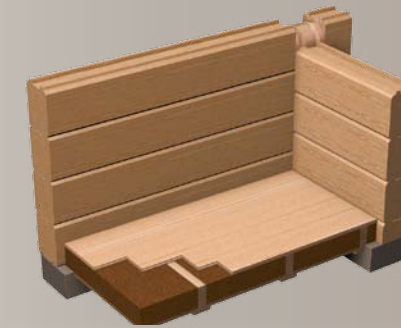
Massive log wall
